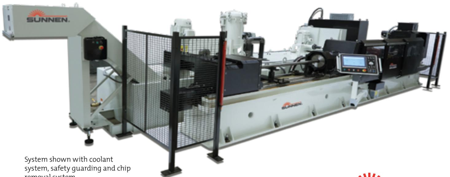
System shown with coolant system, safety guarding and chip removal system.
