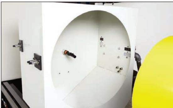
The interlocked rear splash guard incorporates parts present sensors as well as moveable nozzle to deliver honing oil/coolant where needed.
