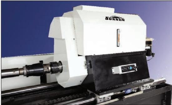
An innovative second station for spindle control ensures one operator can easily do the job of changing driveshafts and setting up the machine.
